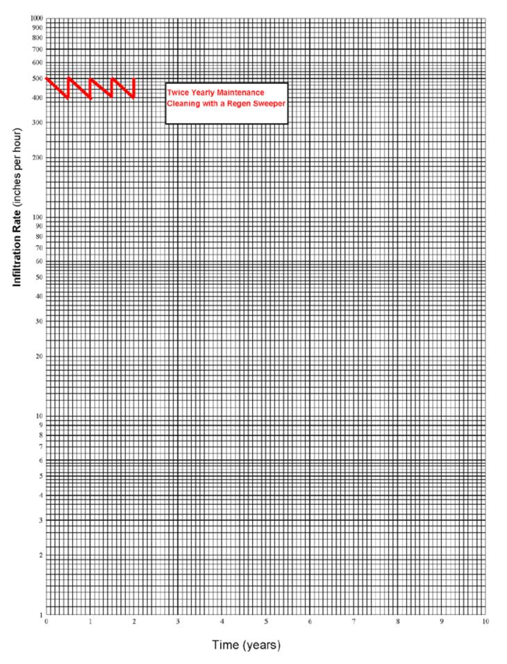
This is a representation of doing routine, biyearly cleaning with a low vacuum regen sweeper. By not allowing the surface to degrade much before maintenance cleaning the full capacity should be retained.
