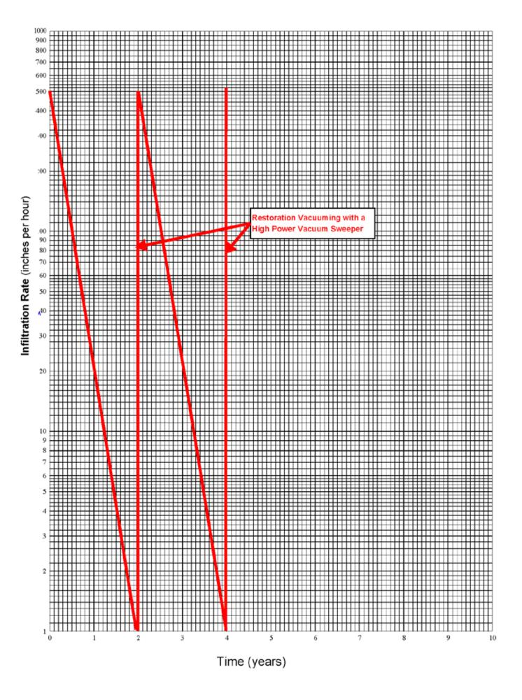
This shows what happens on ICP if it's allowed to plug then restored with a high vacuum source.
